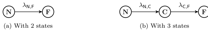
Figure 1.8: Markov chains, where N: nominal behavior; C: non-nominal behavior e.g., due to a crack; F: failure; \lambda is the hazard rate .
